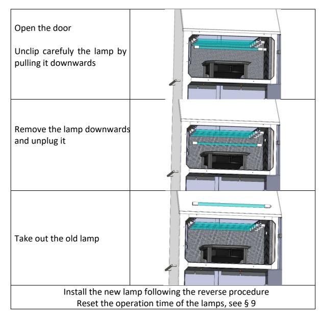
**Warning**: When replacing the UV lamps, take care not to touch the UV lamps with bare fingers, gloves are provided for this step. Cleaning the UV lamp with alcohol will remove all traces of perspiration left by your fingertips.
