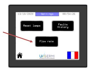
Step 3 : Click on the flow rate to configure box and enter a flow rate between 400 and 1100 m3/h then press OK.
