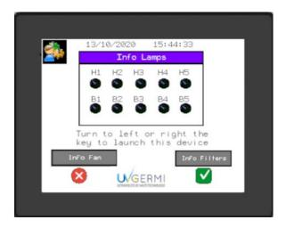
As long as the key is not turned to the right or to the left, the fan and UV lamps remain off.
